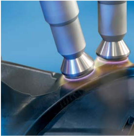
Fig. 3: The robot-controlled, locally selective plasma nozzles eliminate the need for masking when pretreating plastics. (Image Plasmatreat)
