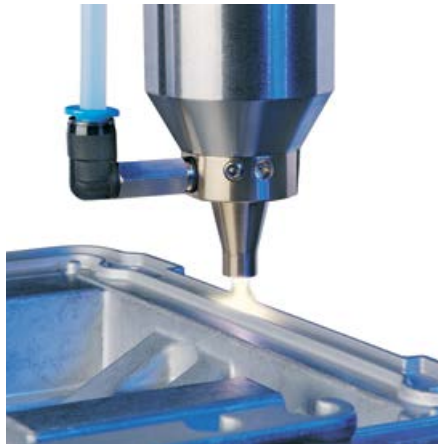
Fig. 4: The anti-corrosive, adhesion-promoting layer deposited with the aid of PlasmaPlus technology not only confers a high level of corrosion protection, it also provides an excellent substrate for many adhesives. (Image Plasmatreat)
