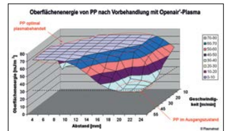
Fig. 2: The figure shows a non-polar plastic surface that was pretreated as a function of distance and speed with plasma. Treatment renders the surface polar and the surface energy rises to >72 dyne with a large process window. (Image Plasmamatreat)
