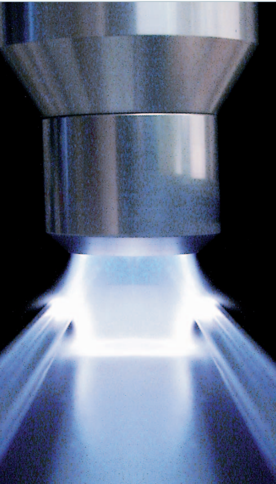
Fig. 1. The electrically neutral open-air plasma beam facilitates micro-fine cleaning, high activation and extremely thin coating of surfaces
